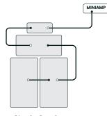
Single Stack Wiring example
